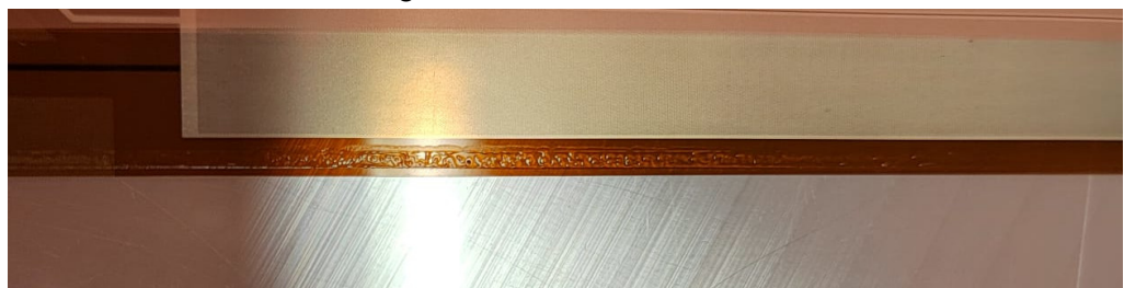
Figure 11: Detail on the glue on the overlap. (This already has too much glue)
