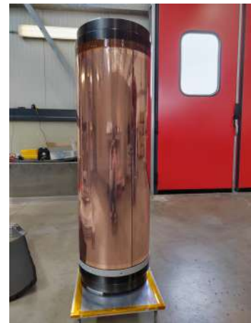
Figure 10: Dressed mandrel on the vertical base
