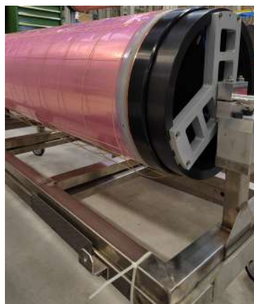
Figure 5: Dressed mandrel secured on the cradle
