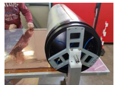
Figure 6: Mandrel secured on the table for cylindrical gluing
