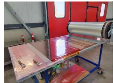
Figure 36: Cilindrical table ready for cylindrical gluing
