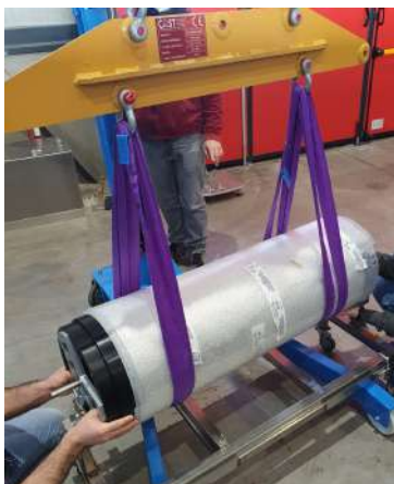
Figure 4: An example on how to hold the naked mandrel
