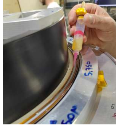
Figure 51: Gluing procedure with syringe
