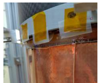
Figure 49: Mylar patches to help the insertion with the grid
