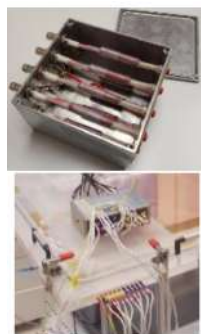
Figure 21: Picture of the HV box for the HV test.
