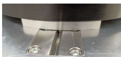
Figure 8: Mandrel centered with the reference pin
