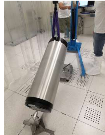
Figure 9: An example of the procedure to raise the mandrel in vertical position
