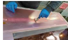
Figure 27: Glue rolling on the vacuum foil patch for transfer
