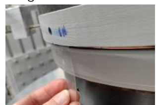
Figure 50: Check during insertion with a thickness the space between the rings
