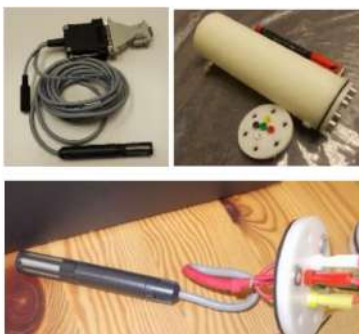
Figure 20: Picture of the HV test table hygrometer system.
