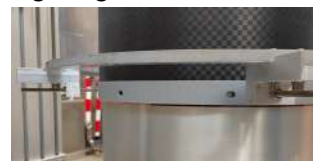
Figure 48: Element extraction with a good point of view on the pushers needed to hold the bottom ring
