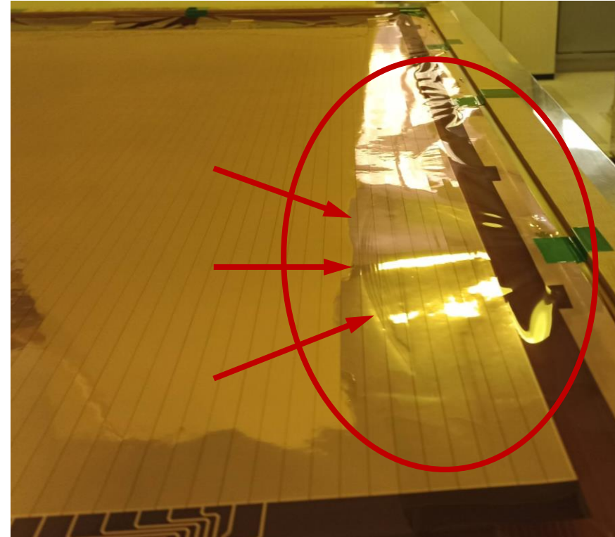
Rejected GEM foil with visible deformations
