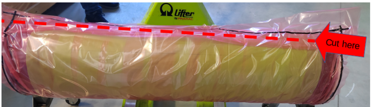
Figure 8: First cut to be done along the length close to the mastic sealant
